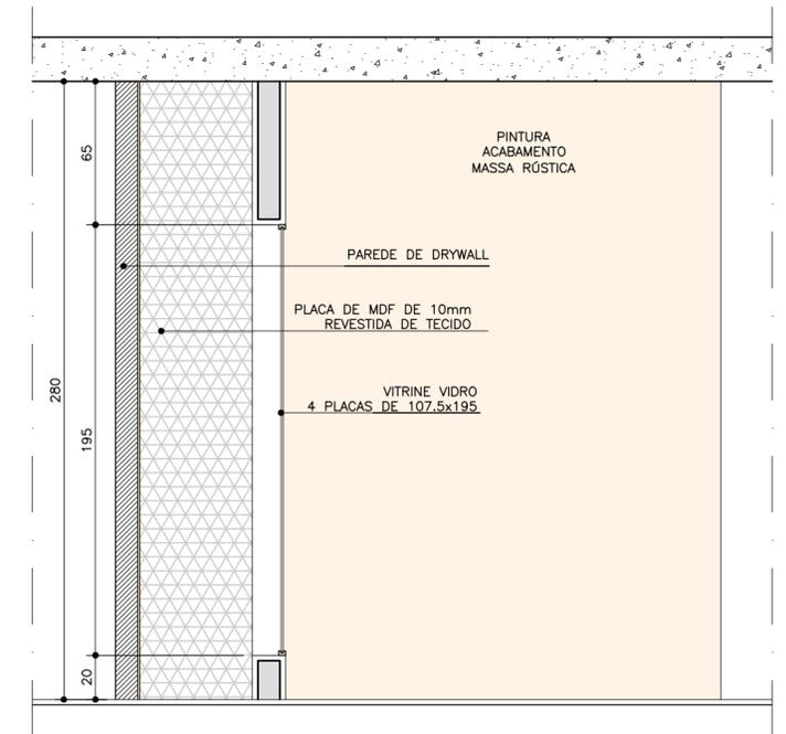
PAREDE DRYWALL . CORTE AA
